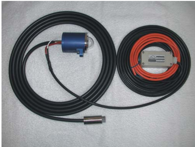
Figure 2 View Global Optic UV-J1002-REG with Light Guide and Temperature Controller
